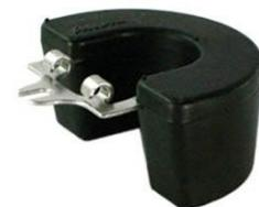
The other was to 'tweak' the tangs on the float. However, the plastic has 'position-memory', returning to its original shape. In tests we found that the tangs loose about 50% of their adjusted position over a four day period, while in a couple of weeks they reverted fully to their original shape. For effective adjustment the 'Stay Up' float is recommended.
